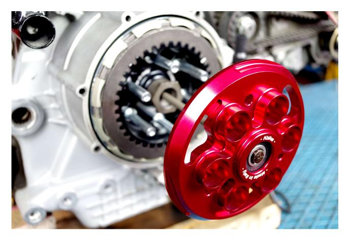
The reference point in the pressurplate must match whit the clutch drum line
